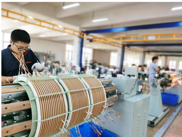
Rectifier transformers winding
